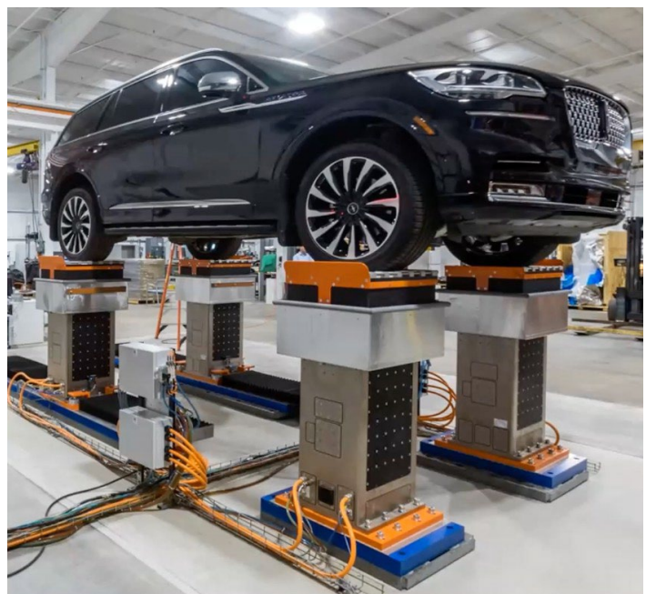
The 4-poster road simulator from eMpulse Test Systems uses servo-electric actuators shown here to simulate road and driving conditions to uncover "buzz, squeak, and rattle" (BSR) issues as well as to assess the noise, vibration, and harshness (NVH) characteristics of vehicles.
