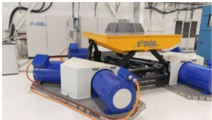
The seaMast shaker table from eMpulse Test Systems uses six to eight servo-electric actuators to simulate diverse vibration conditions. This testing equipment is designed to test specific components such as seats, instrument panels, sub-systems, and more.
