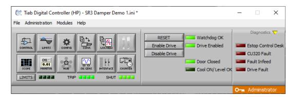
When used in conjunction with M10 Fatigue Test Software, BL1 Generic Purpose software can provide a convenient method to Install, Tune, Configure, Setup Upper and Lower Peak Limits, Run, Monitor, and Collect Data on many endurance or Durability test configurations.
